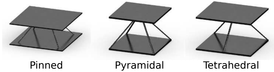
Fig. 1. Unit cells of each configuration with the foam removed for clarity.
