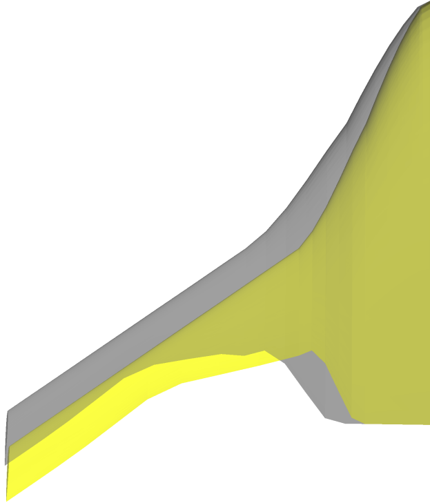
Fig. 12 Comparison of optimized BWB planform geometry. The gray is the MDO result and the yellow is the MDOUU result.
