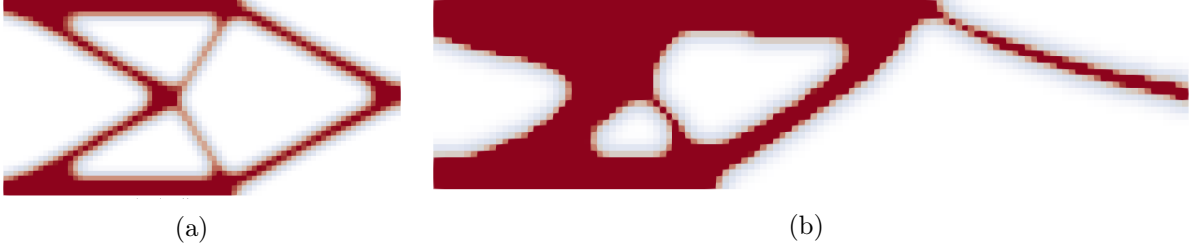
Figure 6: Topology optimization of linear and nonlinear cantilever-beam compliance minimization problems. (a) topology optimization results with a linear elastic model; (b) topology optimization result with a nonlinear neo-Hookean model.
